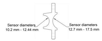
This two-sided sensor retainer can be used for varying sensor diameters depending on which side of the retainer is being used.
